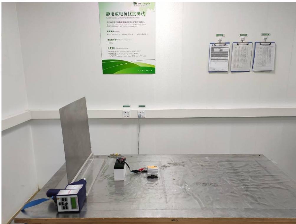
Test Setup Photo of Electrostatic Discharge Test
