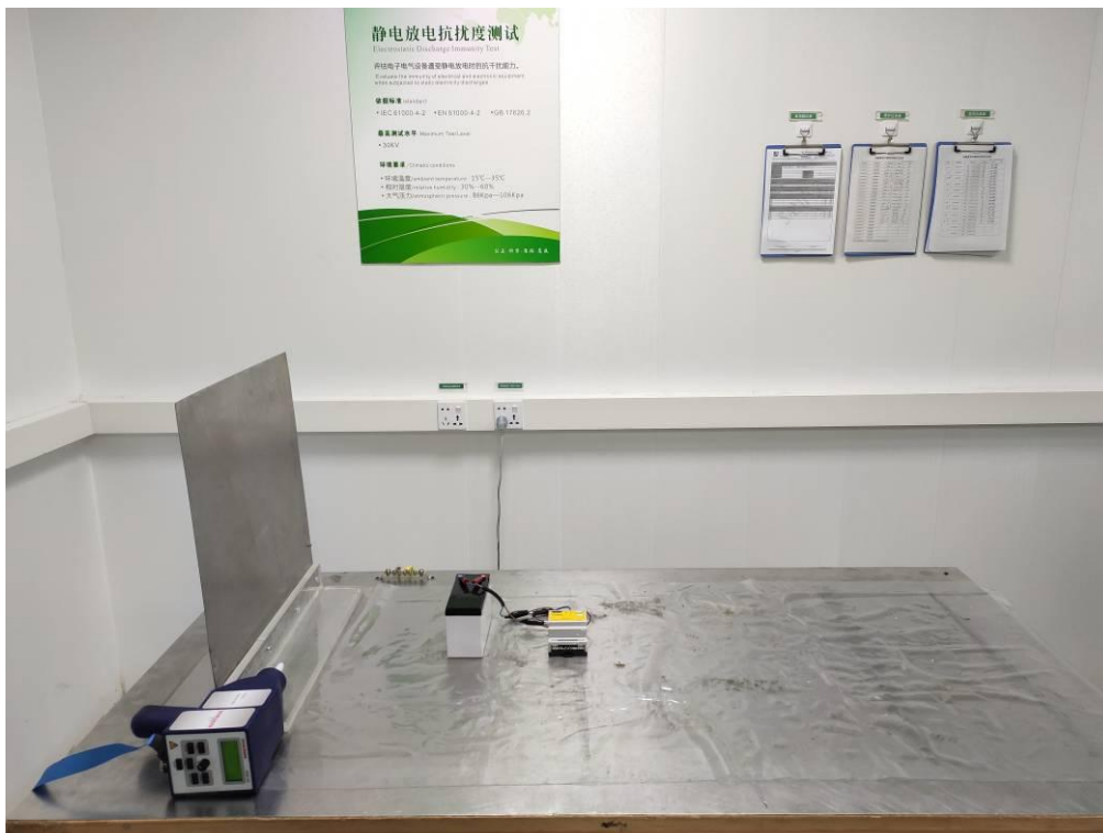
Test Setup Photo of Electrostatic Discharge Test
