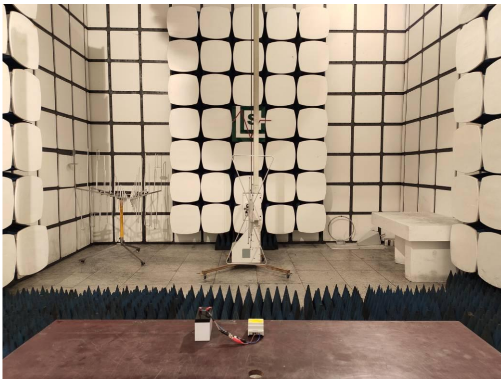
Test Setup Photo of RF Electromagnetic Field Measurement
