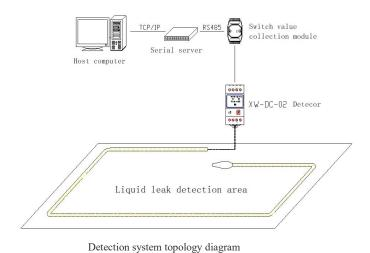
XW-DC-02 Simple leak detector connect with sense cables, and the leakage data can be collected through the switch value collection module and uploaded to the host computer. Sensor relay output signal can be used to control peripheral equipment such as acousto-optic alarm, telephone dialer, SMS module, switch value collection module, etc.
