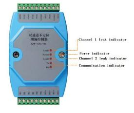
Install the detector in a secure indoor collection box or cabinet where it is easy to maintain and check. Avoid high temperature, high humidity, vibration, corrosive gases, and other electronic interference sources. The detector buckle is mounted on a standard 35 mm DIN rail.
