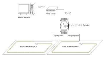
Detection system topology diagram
